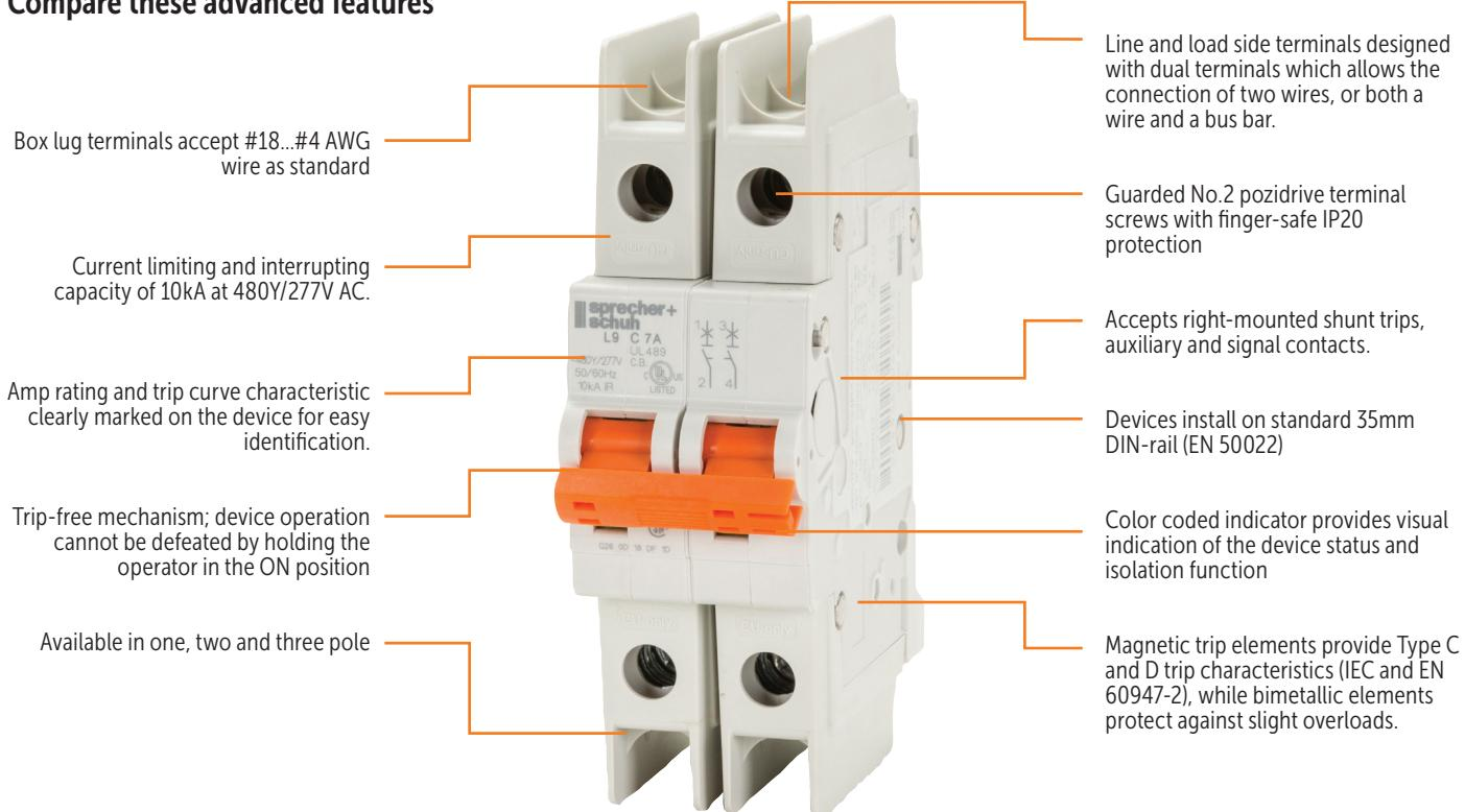
**Trip Characteristic C ( $5 \sim 10 \times I_N$ ) – Inductive loads**
