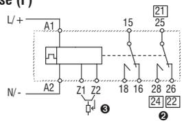
**On-Delay Pulse Generator (I)**
