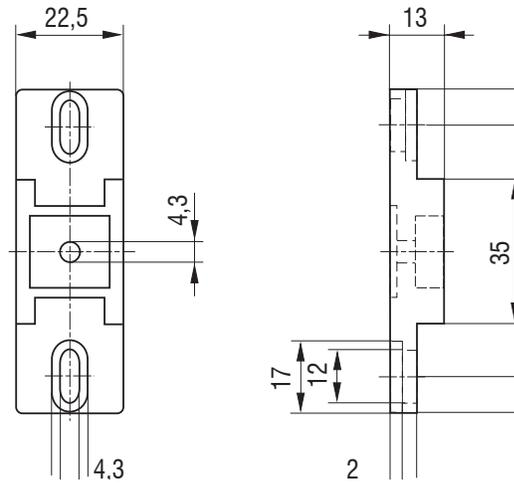
**Series RZ7-FE Timing Relays (one and two pole)**
