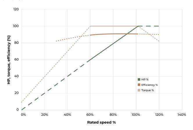
Note: Infinitum does not recommend using the motor below 60% of rated speed except when coasting or ramping up. It is also essential to restrict power and FLA within the nameplate rating when operating the motor above 100% of its rated speed. To operate the motor outside the recommended operating range, please contact the factory and our Application Engineers will provide a customized solution.
