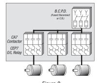
Figure 2 NEC Article 430-53 circuitry without KT9/KT7
