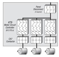
Figure 7 Multi-motor Starter Panel using KT9 as Type E Combo Starter (BCPDs) per NEC Article 430-52 (c6)
