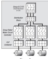
Figure 8 Article 430-53C Circuitry With Group Rated Controller
