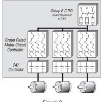
Figure 3 Article 430-53C Circuitry With KT9, KT7, KTA3, KT4 or KT5
