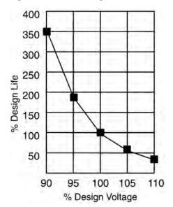
Figure 2. Effect of Voltage on Life of Incandescent Lamps
