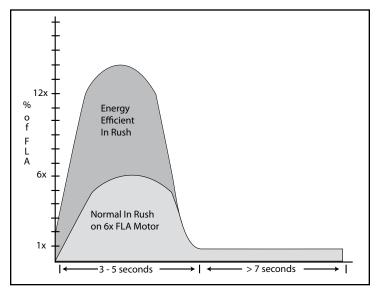
**Figure 2: Typical Motor Inrush**
