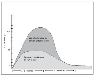
**Figure 3: High Efficieny Motor Inrush**
