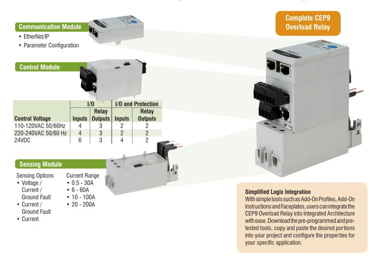
Trip adjustments include a trip setting adjustable from 50...600% FLA and a trip delay time with a range of 0.1...25 seconds. A separate warning setting is adjustable from 50...600% FLA.
