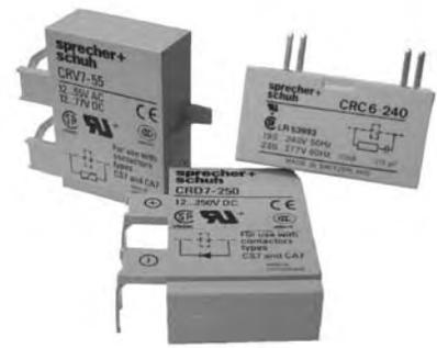
Surge Suppressors are used to suppress the high voltage spike that is generated when a relay or contactor coil is de-energized. The electromagnetic field collapsing across the coil generates a voltage spike in the wires of the control system. Without the suppressor, the surge can reach 8 to 10 times the rated coil voltage and can propagate through the system causing electronic controls to go to unwanted states and filling counters with erroneous numbers.
