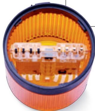
Different individual modules require different numbers of contacts. The new inner contacting offers 8 contacts, which enable a total of 7 positions. This makes challenging, visual-audible tower variants feasible. The unique and patented inner contacting also enhances the visual appearance of the PC7, as the externally visible contacting wires that were previously used are no longer required.
