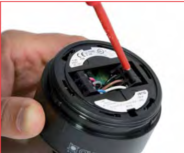
Screwless terminal connection (ECOmodul 60 and 70)
