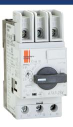
Sprecher + Schuh's KT7 motor circuit controller combines several control and protection functions into one compact unit. It provides Class 10 thermal overload protection, current-limiting short-circuit protection up to 65kA, and signaling capabilities. And its rating as a self-protected Construction Type E device allows it to serve as the motor disconnect, and eliminates the need for additional circuit breakers or fused disconnect switches to provide branch circuit protection.
