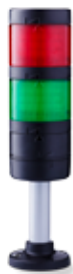
Order no.: PC7-Q02 Colours: red/green Function: LED steady beacon Nominal voltage: 24 V AC/DC Type of mounting: Tube mounting (100 mm | 3.94 inch tube length)
